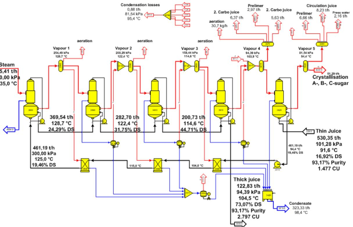
Figure 2b: Flow diagram of evaporation in modified process variant
