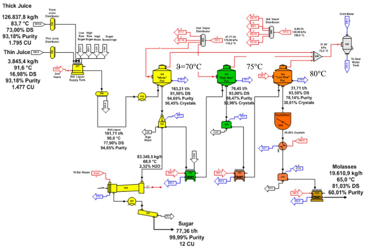
Figure 1c: Flow diagram of crystallisation in basic process variant
