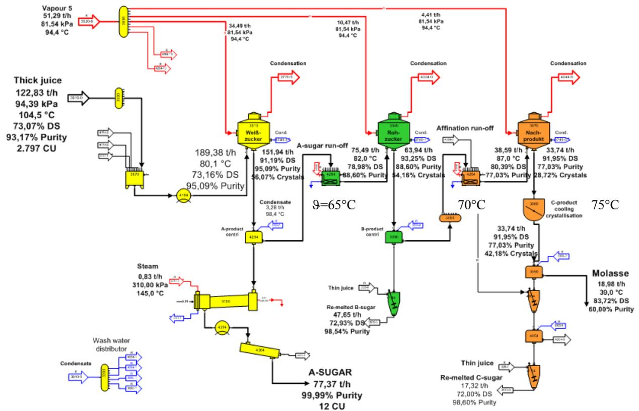
Figure 2c: Flow diagram of crystallisation in modified process variant
