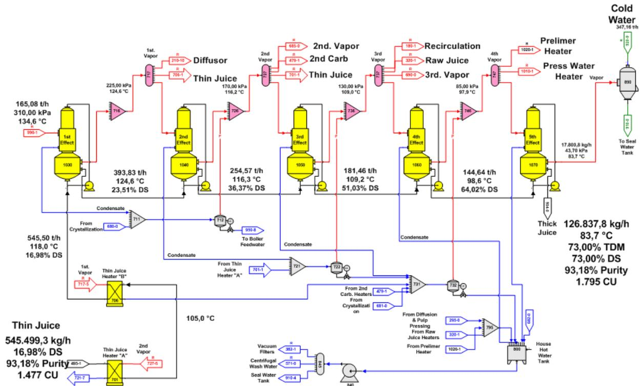
Figure 1b: Flow diagram of evaporation unit in basic process variant
