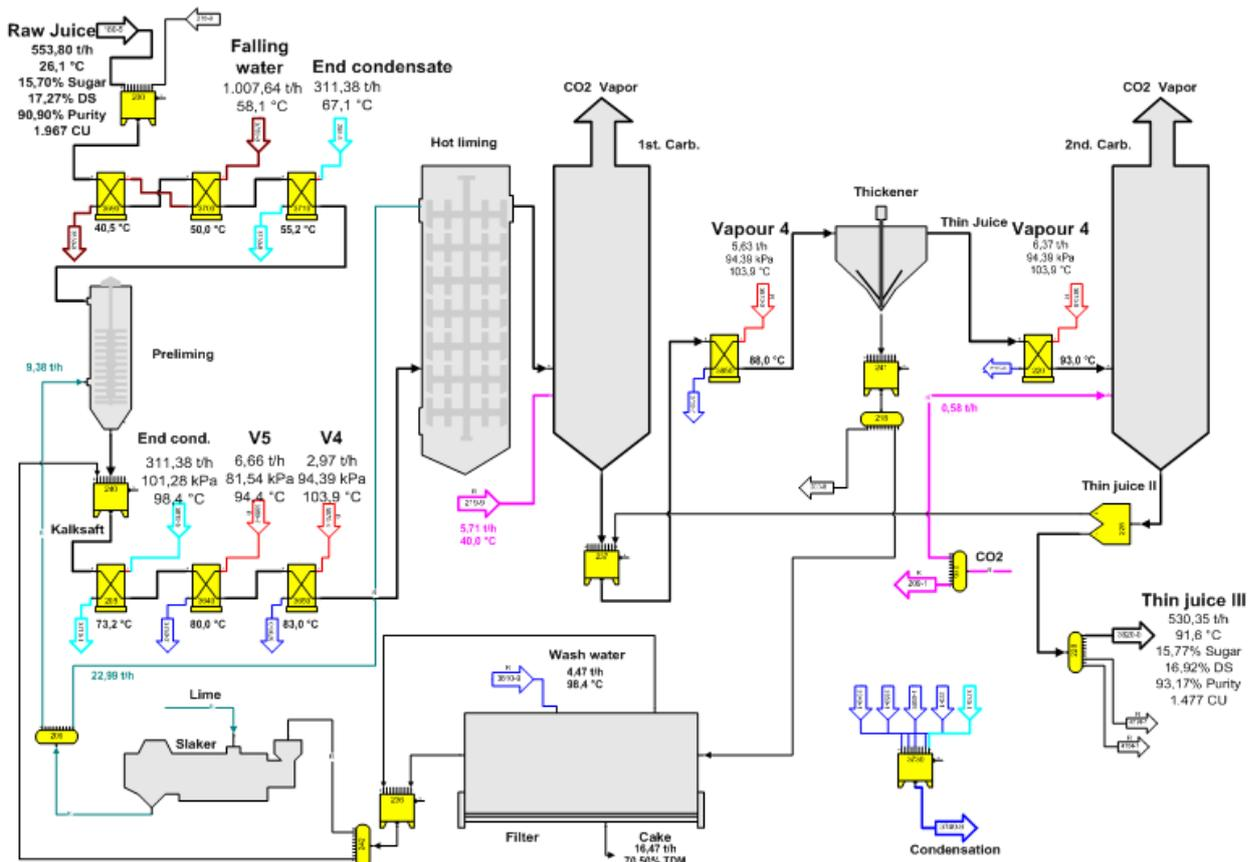
Figure 2a: Flow diagram of juice purification in modified process variant (V4,5 = vapour 4,5)
