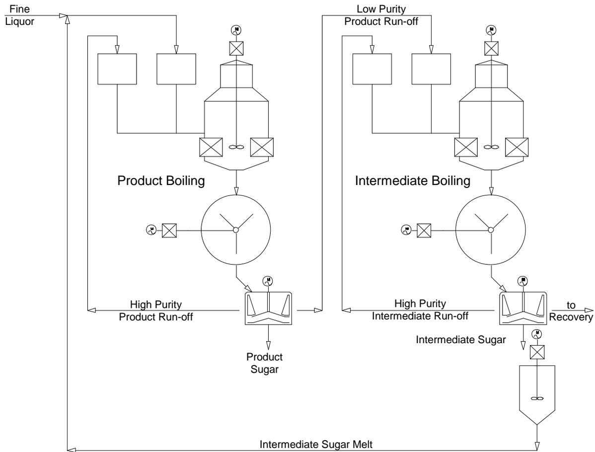
**Figure 1 : The Front End Boiling Scheme**
