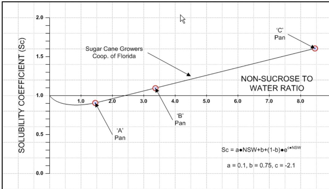
Fig. 2 - Solubility coefficient vs. non-sucrose to water ratio
