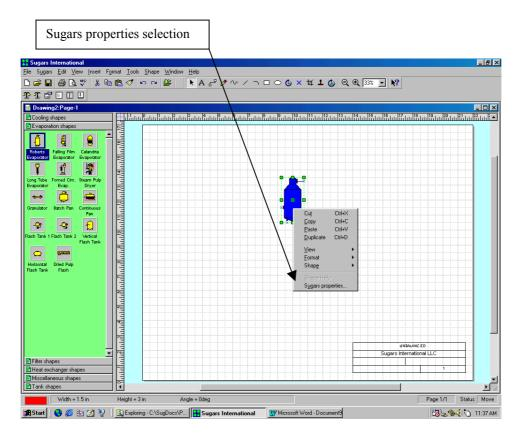
The shape color turns to blue after the station number is entered. Double click the shape (or right click and select "Sugars properties" from the drop-down menu - see figure above) to get the data entry screen (Evaporator Properties screen in the figure below).
