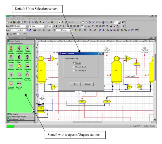
The above figure shows the Units Selection screen for selecting the system of units to be used with Sugars for entering data and displaying the results from the balance calculations. The default system of units is used when a model is saved, even if the displayed units are different. Units are available for SI, US with temperature in °C and US with temperature in °F systems.
