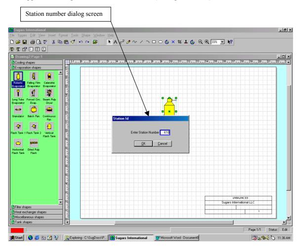
The station number for each station in a model must be unique. Sugars will automatically index the station numbers by 10 as each new one is added to the flow diagram; however, the number may be changed on the dialog screen to any unused number in the model.
