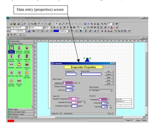
All of the necessary data to describe the performance of the station is entered on the Properties screen. The station turns yellow to indicate that data for the station was entered after the Properties screen is closed by clicking on the OK button. Shapes are added to the drawing until all of the stations for the model are on the drawing and data is entered for each station until all of the stations in the model have turned to yellow.
