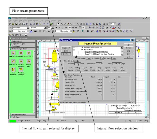
Every internal flow in the model can be displayed using the Properties screen. Also, flow streams that are required and/or pressure feedback (flow streams that need a pressure value from another station) are identified on the flow diagram by a small 'R' for required and a small 'P' for pressure feedback. Sugars will place these indicators on the flow streams after the balance calculations are completed.
